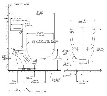
NOTES: THIS TOILET IS DESIGNED TO ROUGH-IN AT A MINIMUM DIMENSION OF 305mm (12") FROM FINISHED WALL TO C/L OF OUTLET. SUPPLY NOT INCLUDED WITH FIXTURE AND MUST BE ORDERED SEPARATELY
